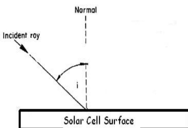
A student wishes to determine if changing the **angle of incidence** of sunlight throughout the day affects the voltage produced by a solar cell.
