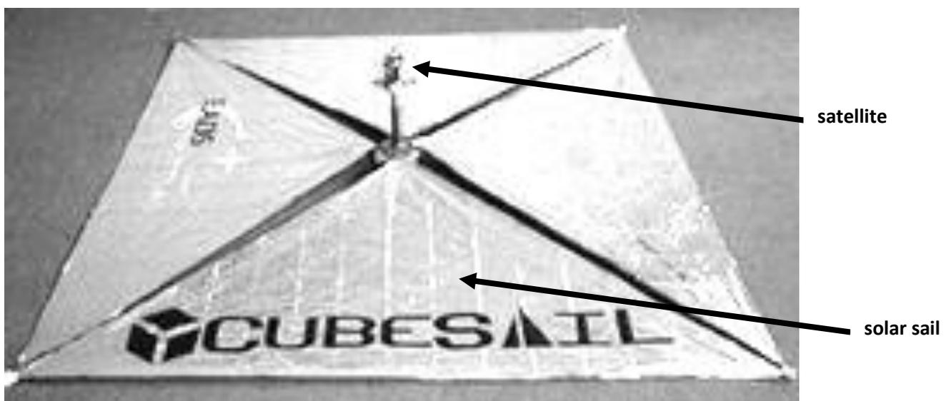
A **prototype** of Dr. Lappas' design, called CubeSail, will be launched late next year. It weighs just 3 kilograms and, when folded up, measures 30 cm by 10 cm. Once **unfurled**, however, the sail will have an area of 25 m<sup>2</sup>.
